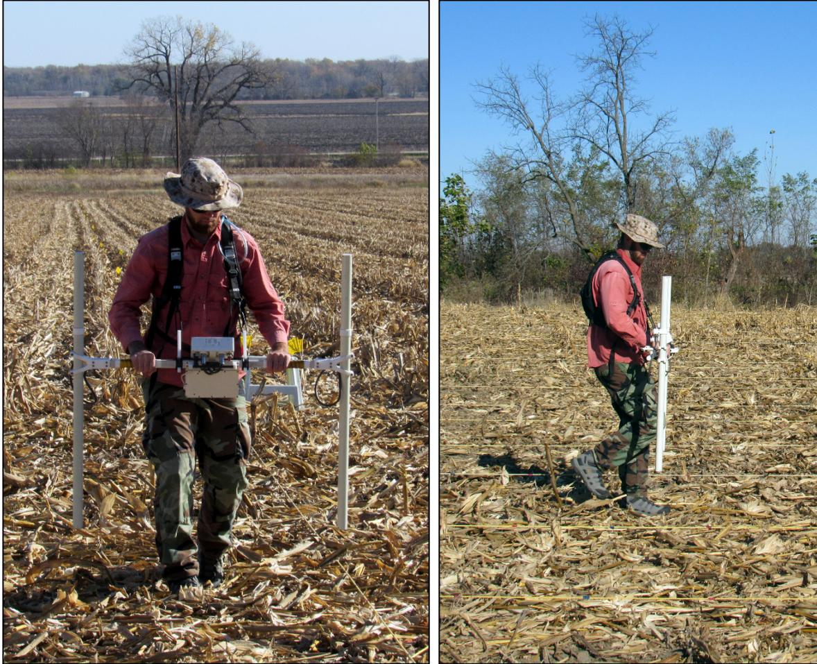
Figure 7. Bartington Grad601-2 fluxgate magnetic gradiometer system in use at Gast Farm. Note the survey ropes used to facilitate the survey effort.
