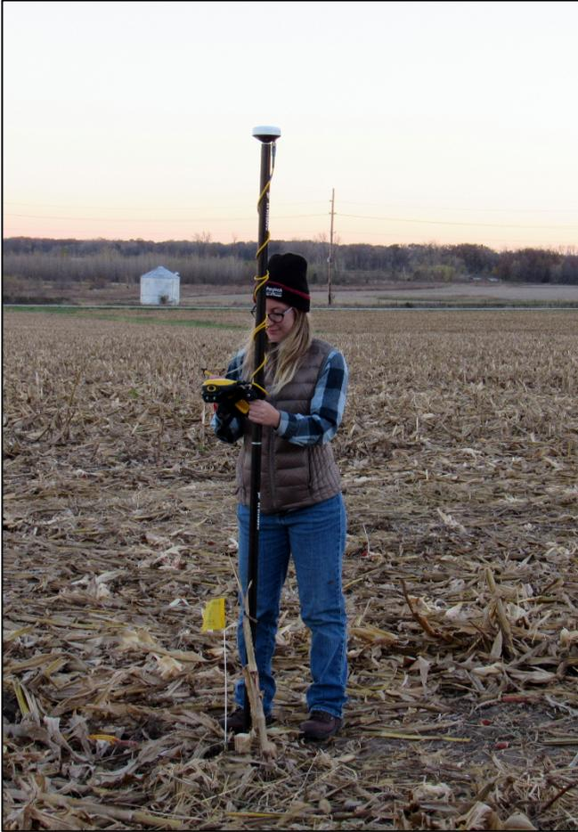
Figure 6. Documenting the locations of survey grid corners with a Trimble Geo 7X and Tornado dual frequency antenna.
