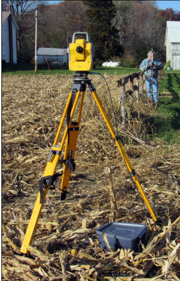
Figure 5. Positioning a backsight point and determining the survey grid orientation with a Ushikata surveying compass (left) and recording the backsight location with a Trimble 5500+ robotic total station (right) at Gast Farm.
