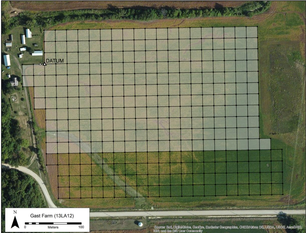
Figure 4. Geophysical survey area at Gast Farm with 297 complete 20-m-x-20-m grids. The shaded area illustrates the portion of the field in which the survey was completed (Aerial photograph source: Esri, DigitalGlobe, GeoEye, Earthstar Geographics, CNES/Airbus DS, USDA, USGS, AeroGRID, IGN, and the GIS User Community).
