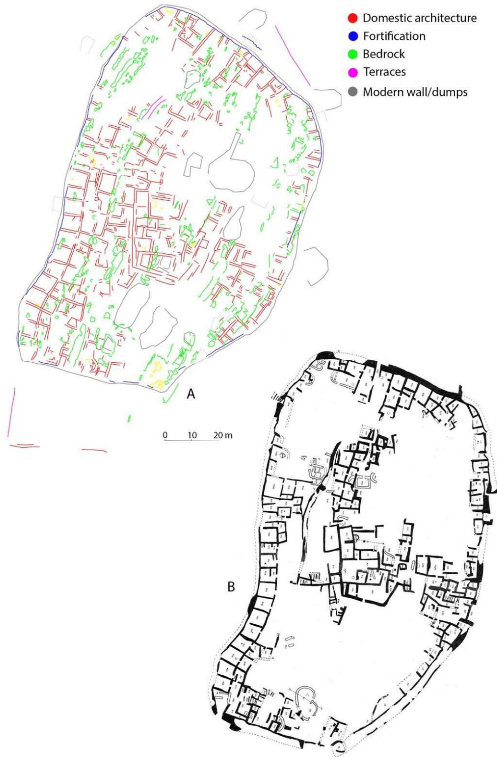
Fig. 2: Comparison of (A) new plan created with a Leica Viva GS14 GPS from architecture remaining in 2015 and (B) plan from 1938 by Natan Valmin.
